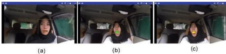
Figure 13. Screenshot of system detection result: (a) normal condition; (b) mouth open detected; (c) drowsiness recognised.
