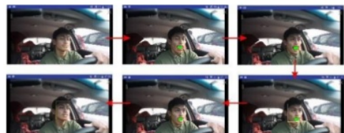
Figure 17. False negative (FN) condition when respondents yawn but no alert shown. Error detection could cause by Haar-Cascade fails to detect face because there are things on driver's face, or respondents yawn under 5 seconds.
