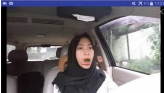
Figure 9. Screenshot of system view. The green line is the contour and the red-rectangle around the contour is bounding box (bb) contour.
