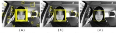
Figure 2. Illustration comparison of detection results with modified minNeighbours: (a) value 0; (b) value 3; (c) value 8.
