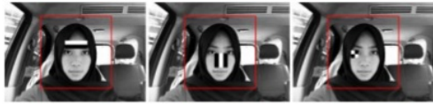
Figure 1. Illustration of the grayscale frame with red-box sliding windows with haar-like feature inside.
